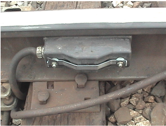
Transducer mounting using Locking fasteners
