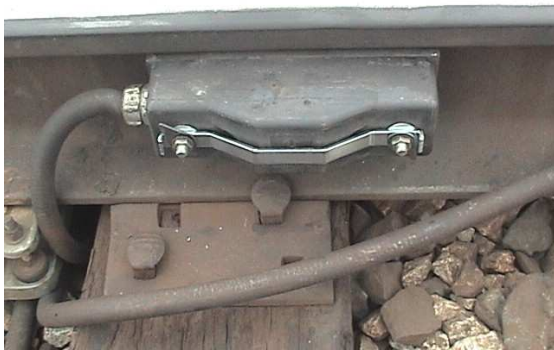
Transducer mounting using Stage 8 fasteners
